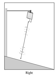
The JC Depth Sensor must be mounted perpendicular to the target surface. Mounting the sensor at an angle will result in erratic and unreliable measurements. To improve the accuracy of the sensor measurements, mount the sensor as close to the target as possible. This will minimize errors that are a percentage of the distance measured. However, the sensor can not measure closer than .5 meters to the target, and should be mounted at least 1 meter away from the target.
