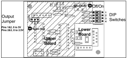
JC Depth Sensor circuit board assembly
