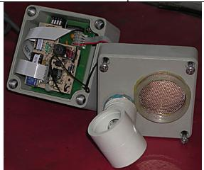
1. Open sensor by loosen the 4 captive screws. Carefully remove the old desiccant pack and replace it with the new one provided. Tuck the new pack in as far as possible so that it is out of the way.
