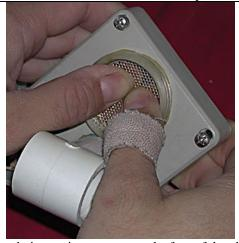
2. Apply increasing pressure to the face of the old transducer with your thumbs until it pops free. Remove any remaining silicone rubber from the sensor case.
