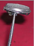
4. Gently lock the forceps onto the plastic tab of the new transducer shown above.
