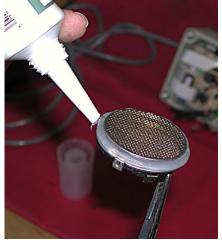
5. Apply a bead of silicone seal to the rim of the new transducer. Avoid getting silicone seal on the grill or terminals. Mount the transducer into the case. Seat the transducer by pressing on the plastic rim only, do not push on the center.
